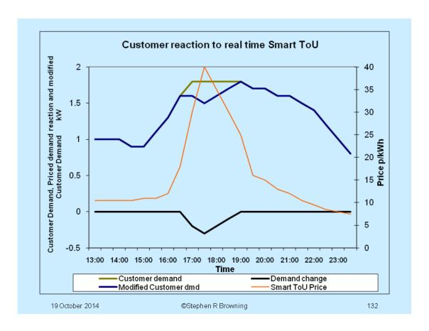
So, this scenario shows the 'Real Time ToU' tariff in action which is all that a lot of existing Smart meters appear to be designed to display.
